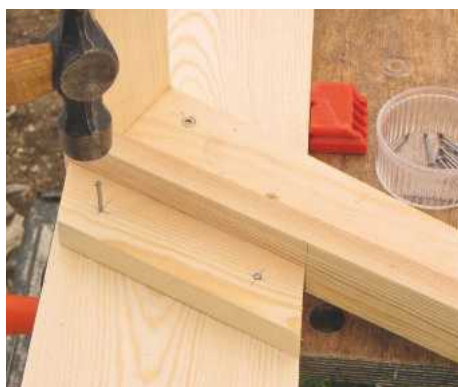
22 Shelf trays are supported by battens fixed to uprights; cut these to length, glue and nail
