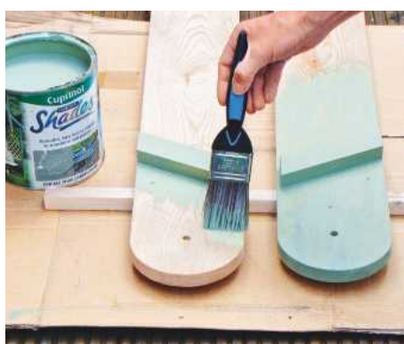
29 Brush on two coats of exterior paint; this is easier to do when the parts are disassembled
