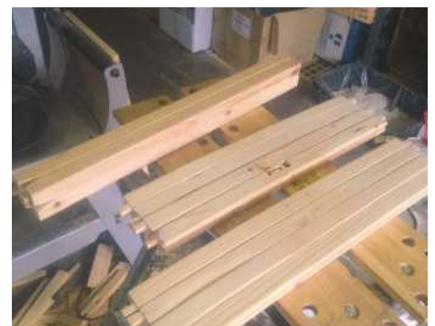
35 Several curves will be applied to the frame's pieces to slim down the blanket chest
