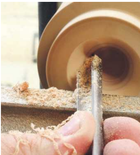
7 Having the wings of the tool ground back allows me to use the tool in a pull cutting mode working from the centre outwards. This will lead to a good surface finish on most timbers
