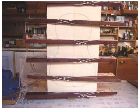
38 The soundboard in the wedge and lace jig
