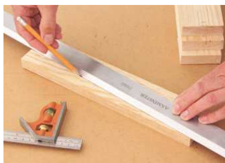
2 Repeat with back rail and draw line between points to create a taper; this will help water run-off
