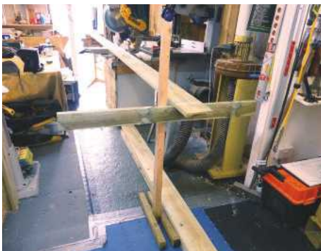
The dead man jig offered support while I was cutting the boards
