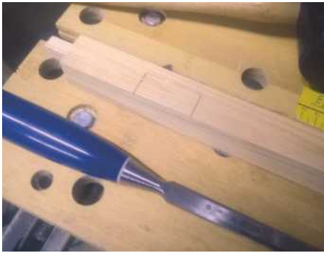
36 Use a utility knife to mark where to make pockets for the hinges to sit into
