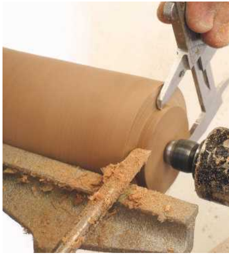
2 Mount the wood between centres and use a spindle roughing gouge to make it round. The box lid and base will both be hollowed, so a chucking spigot needs to be turned on both ends
