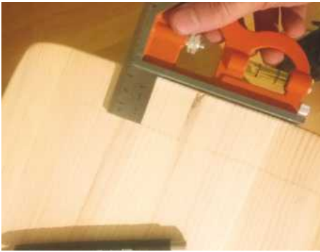
57 Draw the border in pencil by following the edge of the lid with a combination square set to 35mm
