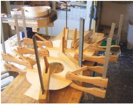
45 The harmonic bars are clamped into place
