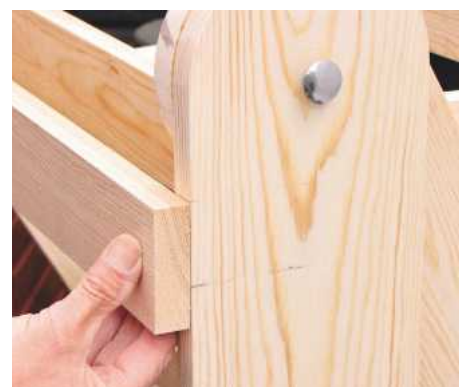
27 If storing the plant ladder over winter, an extra upper stretcher adds rigidity when disassembled
