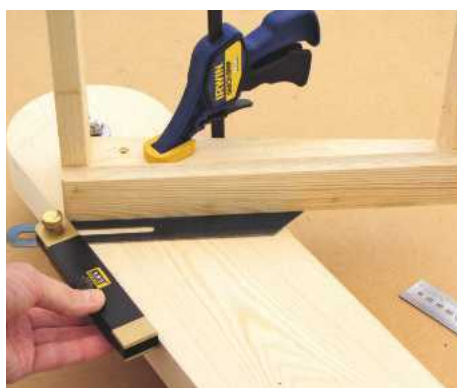
17 Shelves are screwed to uprights at 63°; set the sliding bevel and cramp shelf before fixing
