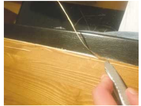
59 I carved a thin decorative V-groove between the black border and the stained part of the lid
