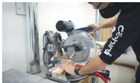
6 Using my mitre saw, I cut the 25mm strips of wood to random lengths
