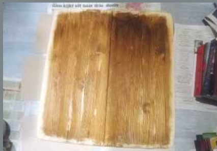
60 Wood stain cannot penetrate glue, so any glue marks can be easily seen when staining wood
