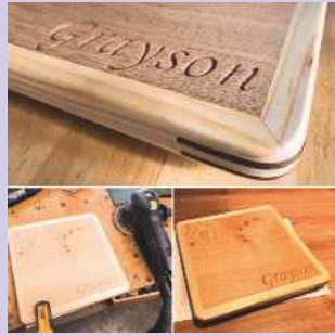
Creating the stool's top, complete with his Godson's name, which was added using a CNC machine
