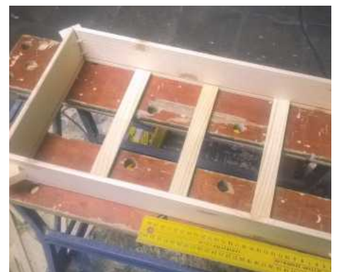
50 To add strength beneath the woven pattern, I cut three slats
