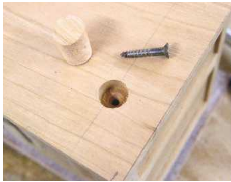
23 Drill holes into which will fit the cherry plugs
