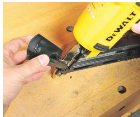
Each gun has a front access area for dealing with nail jams
