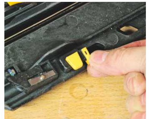
Spare soft-nose tips are supplied and stored on board with each gun
