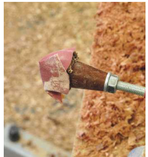
9 Sanding inside a piece like this is never easy with your fingers, so a good method is to make up your own sanding sticks. I'm using a proprietary available sanding ball, which the abrasive is attached to using a hook-and-loop fastening
