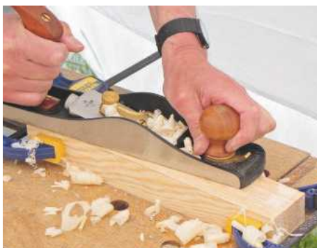
4 Cramp several ends together and secure in a vice; plane down to the pencil line, checking for square
