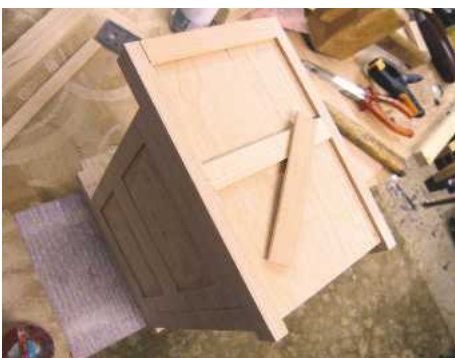
11 Applying the case rails
