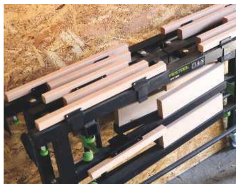
All of the timber components on the STM 1800 are fully replaceable
