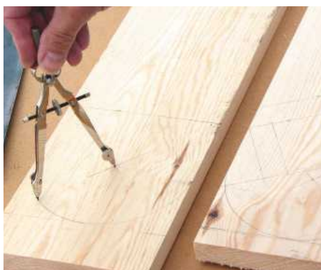
10 Mark the upright to length and use compasses to draw a semi-circular top end on both pieces
