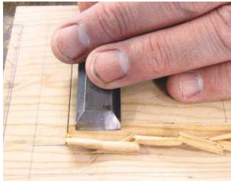
7 Careful work with a chisel will form the bevel
