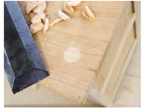
24 The plugs are pushed in and levelled with the top
