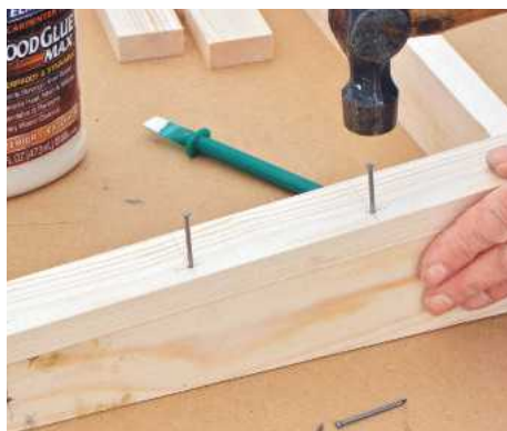
8 Slats are supported by battens nailed underneath the shelves; fix to ends and centre for strength
