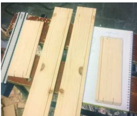
48 To strengthen the mitre joints, I cut two slots in each corner
