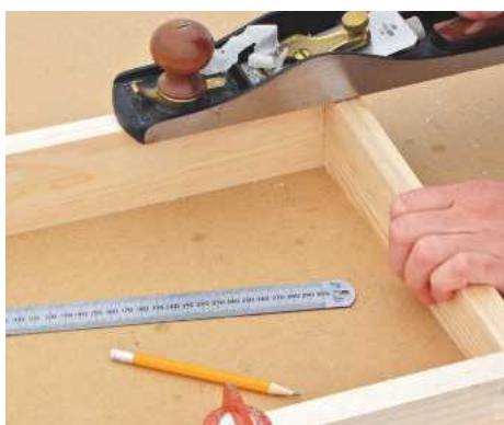
7 Trim the end-grain flush with a block plane; true up top edges with a plane, avoiding breakout
