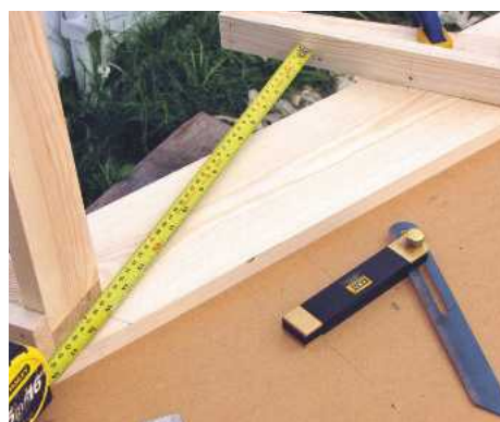
18 Screw upper and lower shelves to uprights first, then check the position of the middle shelf
