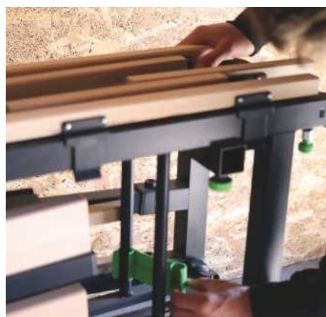
Festool green quick-release lock clasps hold the worktable shut
