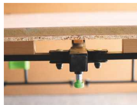
The STM 1800 loaded with a sheet of MDF for cutting and a sacrificial sheet underneath
