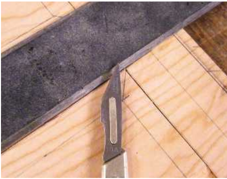
6 A sharp blade slices the wood fibres to prevent tearing
