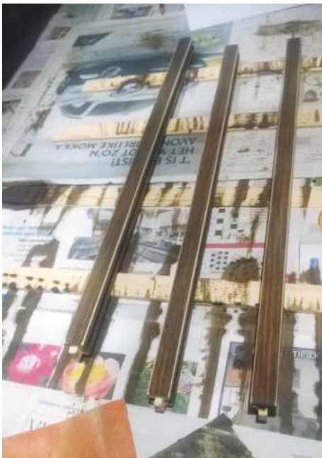
54 You can create a nice effect by lightly sanding the edges of the middle studs, so edges are highlighted
