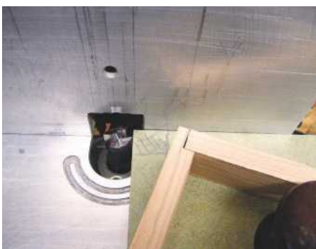
19 Note the MDF support for the narrow timber being cut
