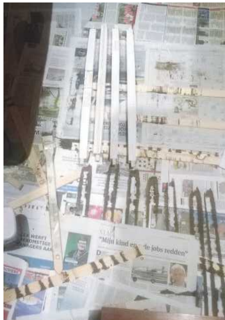
55 Paint one layer of lacquer primer on all frame pieces
