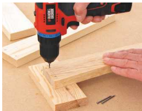
5 Components are simply butt-jointed; pre-drill pin holes to prevent timber splitting when nailing
