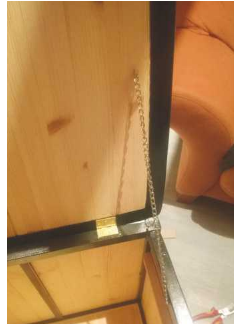
68 Attach a chain to both the lid and frame using two screws and washers
