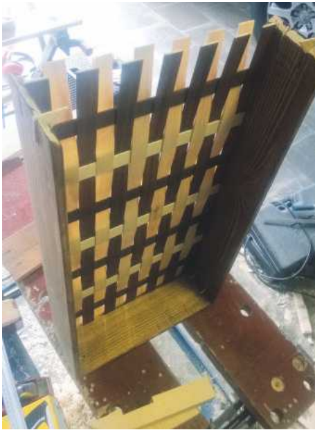
51 I first glued up only two of the mitre joints, together with the strips of wood in their slots
