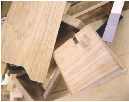
22 Cut a small notch to suit the locking mechanism
