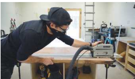
3 Using a large square and my track saw, I cut off the live-edges and set them aside for later
