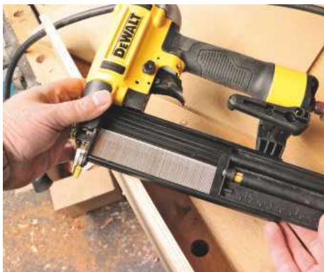
Nails are easy to load; the yellow tab to the right of the nail track indicates if the gun is empty
