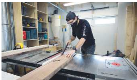
5 Using my table saw, I cut the remaining walnut and the maple into 25mm strips
