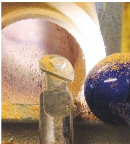
8 If the finish off the gouge isn't as good as it could be, then you may need to reach for the scraper. This tear-drop cutter on a big, solid bar is perfect. Here I'm using an LED light on a flexible stem
