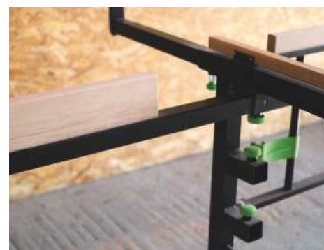
One of the large wooden sacrificial extension support coverings
