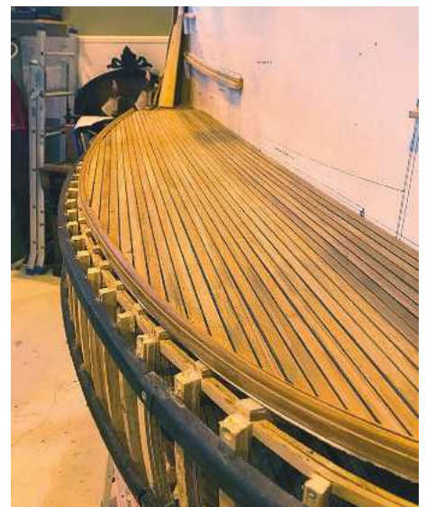
Framing the hull
