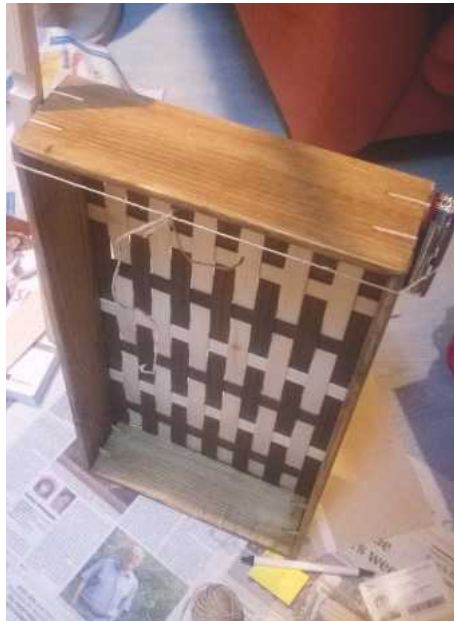
52 I put some clamping force on the sides by tying string around it, and increasing the tension by wedging in a random small object
