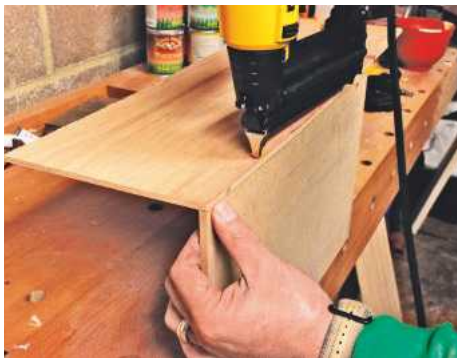
The Precision Point makes it very easy to align on thinner stock
