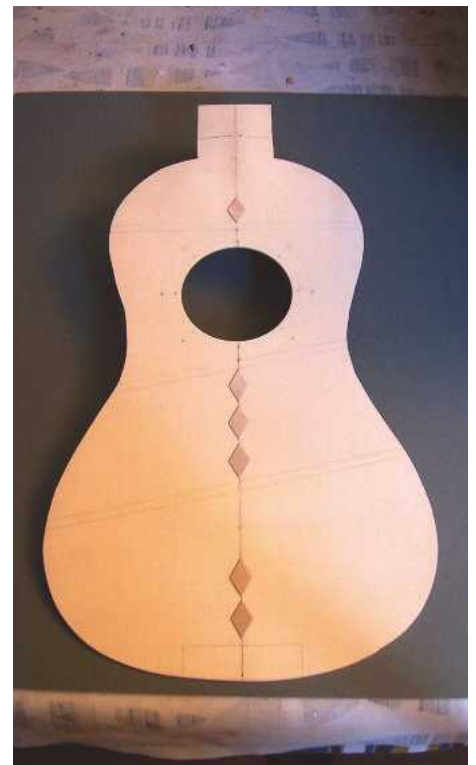
44 Cleats on the inside help to hold the soundboard together
