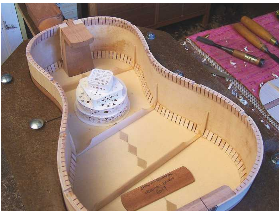
61 The completed rose is fitted
