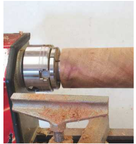
3 You need to decide which end is going to be the lid and this can then be mounted in your chuck. The top of the lid is going to be carved away so if there are any defects in the end of the wood, you will be able to remove them
