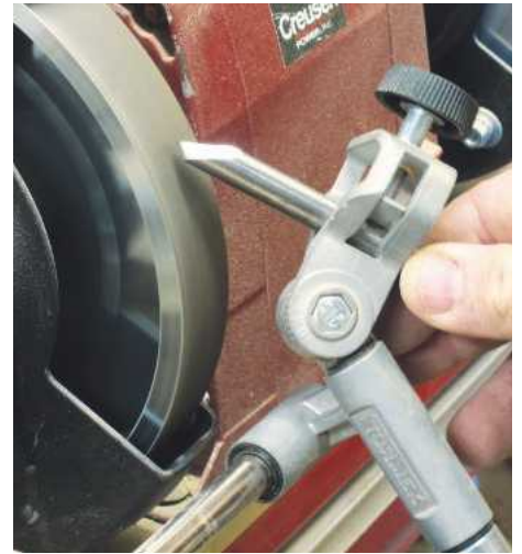
6 My choice of tool for hollowing a box of this size is the 13mm signature spindle gouge. The wings on the tool have been ground back and this is best done using a grinding jig
