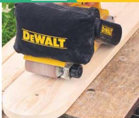
20 Fill any knots or defects in the timber before sanding all surfaces with 120 grit abrasive or finer
