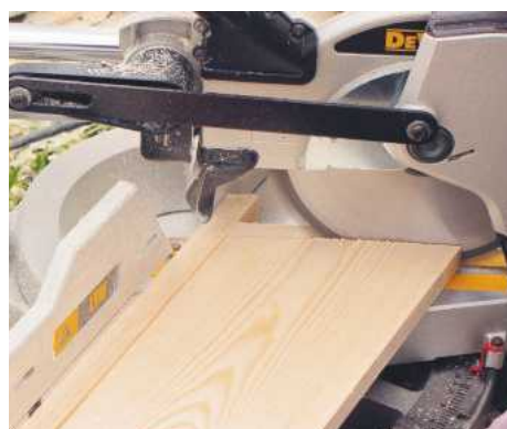
9 Set the mitre saw to 27° and cut the lower end of the front uprights – round off any sharp corners
