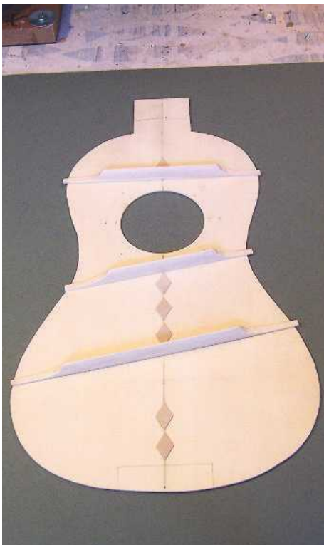
48 The finished soundboard seen from the inside
