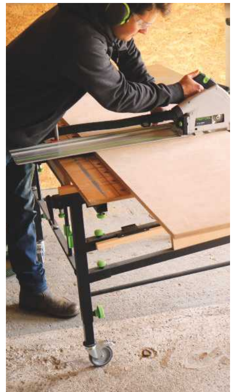
Using the STM 1800 as a cutting station when fitted with a Festool TS55 plunge saw and guide rail
