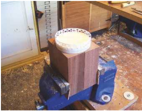
56 A softwood caul keeps the wall in shape
