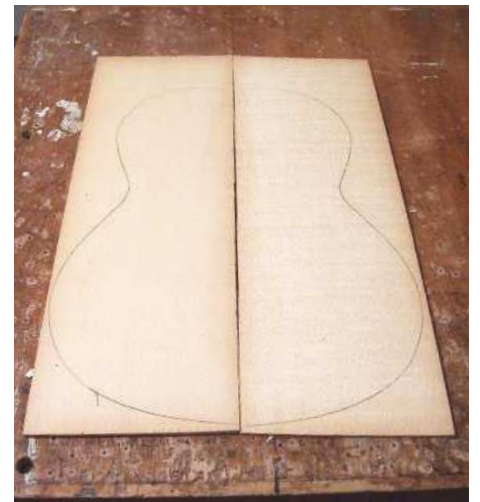
36 A bookmatched soundboard of fine grade Engelmann spruce
