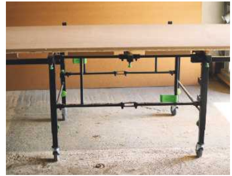
The worktable set up ready for sheet cutting or using as a workstation/assembly table
