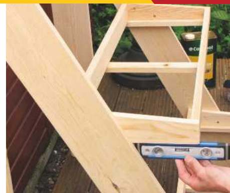
21 To check the length of the rear upright, cramp together and adjust until all shelves are level
