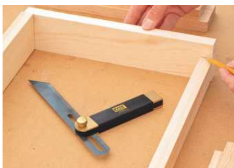
1 Cut shelf ends, front and back components to length; mark height of front rail on end pieces
