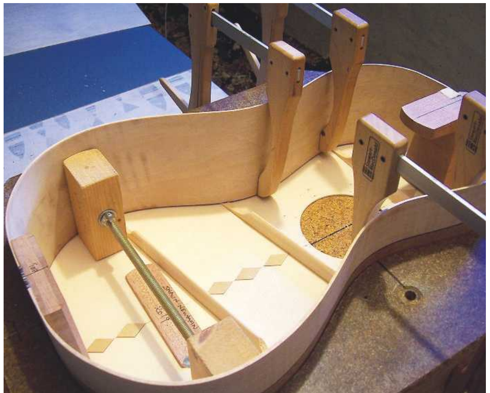
49 The brace ends are marked with a fine pencil line
