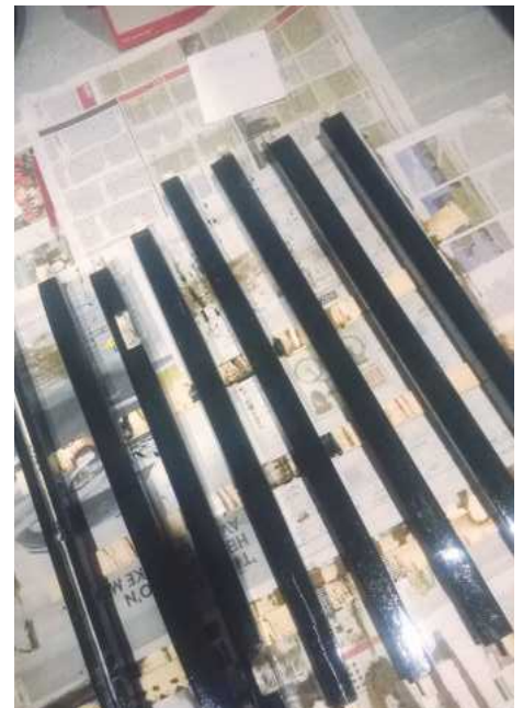
56 Add two layers of black lacquer to the frame, carrying out a light sanding between layers
