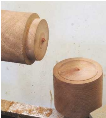
5 When I cut the lid off, I like to leave a tiny piece of the spigot on the base; this will act as a guide to how wide I need to hollow it for a good fit. Remember it's only a guide, though
