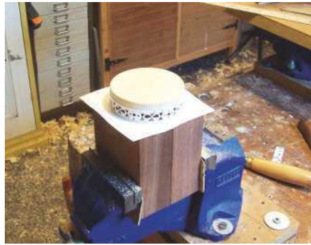
57 The first layer is glued up
