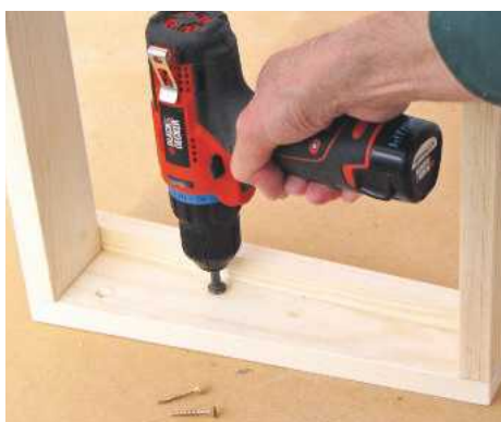
16 Shelf trays are fixed to the framework with 5mm screws; mark hole centres, drill and countersink
