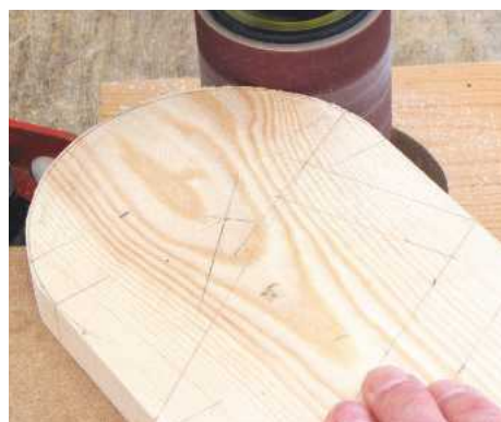
12 Clean up curved ends on a sanding drum mounted in a drillstand; cut rear uprights in the same way
